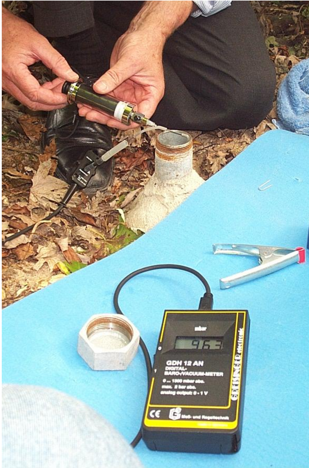
Evacuation of gas from a GASSYS collection chamber by means of a special syringe. Pressure meter in front.
