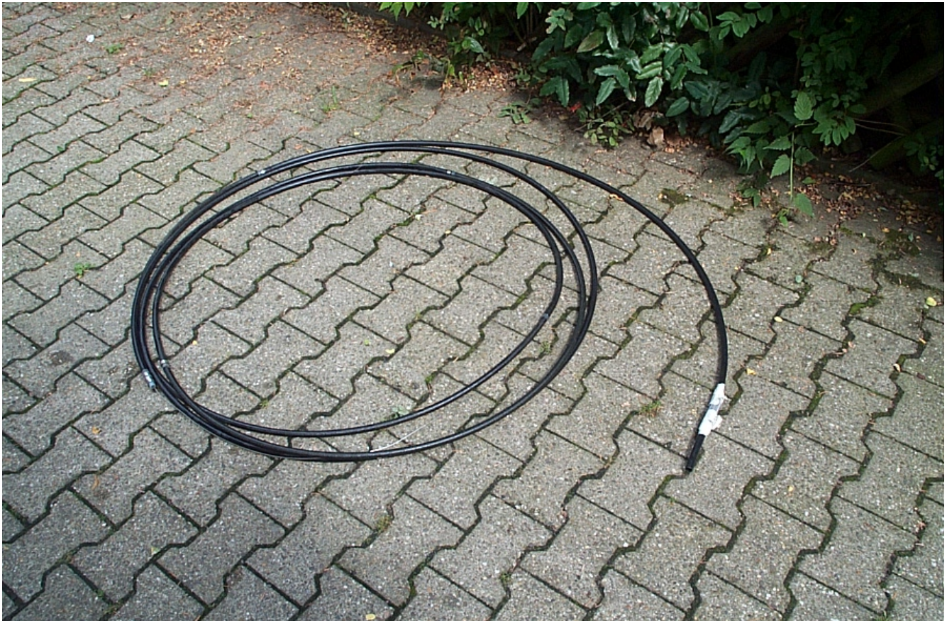
GASSYS hose with two semipermeable collection chambers prepared for installation. The hose system is inserted into the installation casing.
