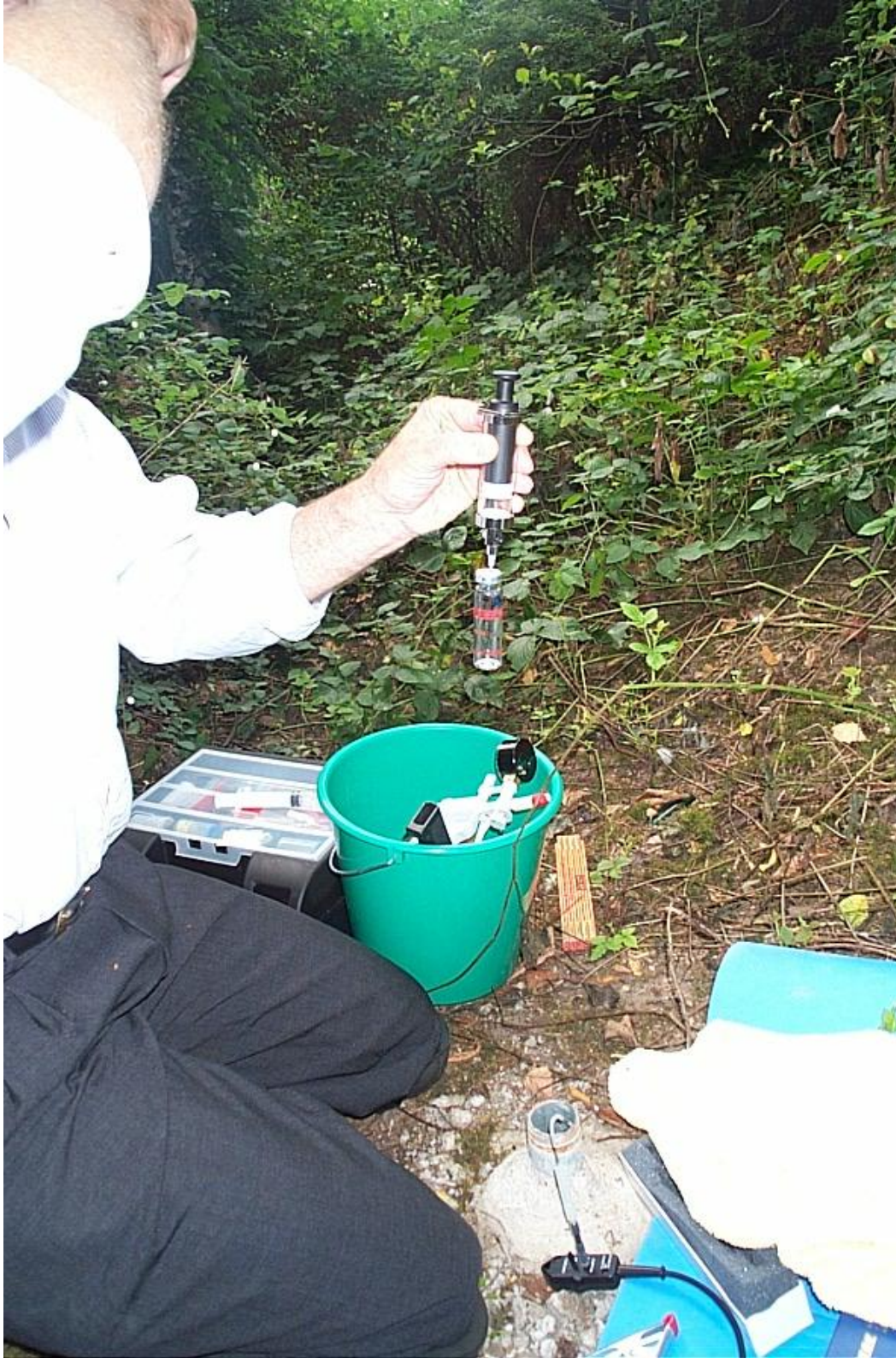
Insertion of gas sample into headspace vial. The sample should be transported to the lab promptly for next-day analysis.
