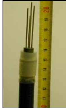
Left picture: Gas sampling system GASSYS with stainless steel tubing connected to four semipermeable chambers. Right picture: Methane measurements in a gas piezometer nest with four chambers at a landfill
